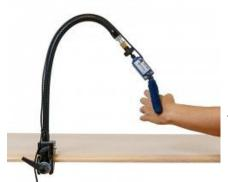
**BJ-B12** Rod switch with a flexo arm
